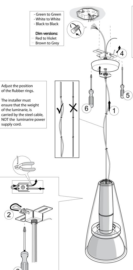
This canopy must be mounted to a standard junction box.
