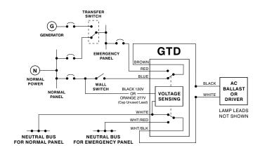
Normal Operation - (Shown Above) AC Lighting Ballast supplied by normal panel & controlled by wall switch. Generator Operation - AC Lighting Ballast or Driver Supplied by generator (or central inverter) through emergency panel and independent of wall switch position.
