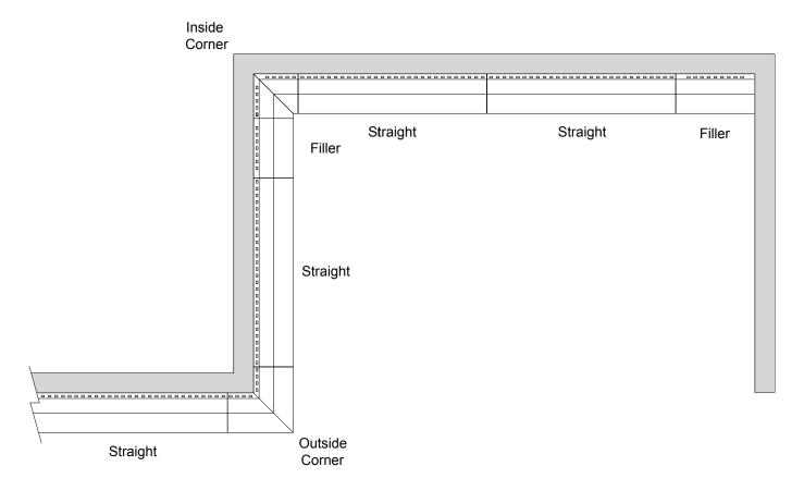
After installing mounting channels around the perimeter, place the corner fixtures, followed by straight fixtures. Trim the filler fixtures to fit remaining run lengths and place onto the mounting channel.
