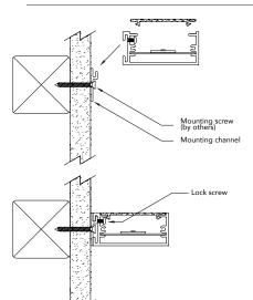
Use appropriate fastener through provided holes in the mounting cleat
