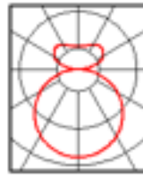
30/70 – Option 3415 lumens 33% up - 67% down 80 lm/W
