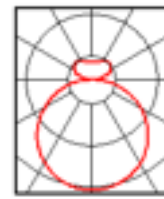
20/80 – Option 3285 lumens 22% up - 78% down 75 lm/W
