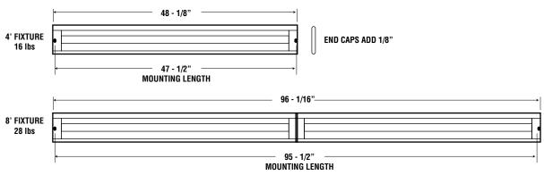
CONTINUOUS ROW CABLE MOUNTING 4' FIXTURE - 4'-1/8" 8' FIXTURE - 8'-1/16"
