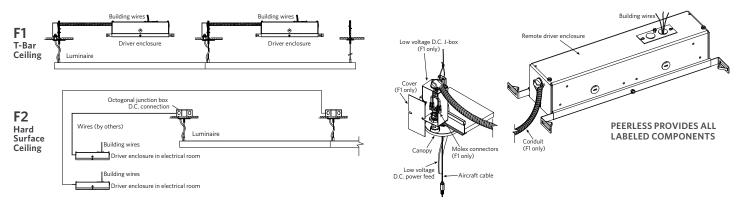
The driver is housed in a remote-mounted, aluminum enclosure. In T-bar ceiling installations, the driver enclosure attaches to the grid bars with provided hanging brackets and clips. For hard ceiling installations, the driver enclosure resides inside an electrical room and can be mounted to a rack or wall with screws (by others), if necessary.
