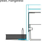
Recessed box allows for 1/2" of adjustability to accommodate a variety of grid ceilings
