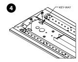
Surface mount fixture to desired location by installing appropriate hardware thru key-ways in the pan.
