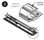
Remove driver cover by removing (2) screws. Set aside.
