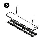
Reinstall the lens by placing the lens over the fixture on one side, then bring the lens over the opposite side.
