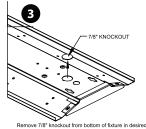
Remove 7/8" knockout from bottom of fixture in desired location to allow for wiring. Bring supply wiring thru and wire in accordance with all national, state and local codes.
