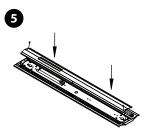
Reinstall the driver cover making sure all wiring is tucked safely under the cover. Test the fixture.
