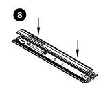
OPTIONAL-PENDANT MOUNT: Reinstall the driver cove making sure all wiring is tucked safely under the cover. Test the fixture.
