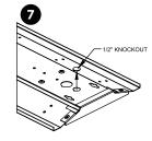
OPTIONAL-PENDANT MOUNT: Prior to Step 5, remove 1/2" knockout from both ends of fixture.
