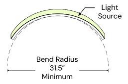
\* LED strip only bends vertically along light surface. Do NOT bend more than the indicated minimum bend diameter (shown above). Doing so will damage the LED strip.
