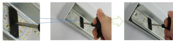
A4. Connect male-connector to female connector on carrier
