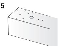
7/8" knockout is located on the back of the fixture to allow for wiring. Bring wiring through.
