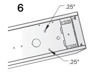
Mount fixture to surface by installing screws through .25" holes (or keyways if applicable) located on back of fixture.
