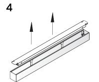
Remove LED assembly (it will hang from tethers) and set aside.
