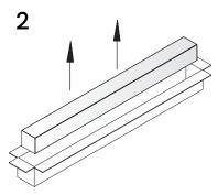
Carefully remove fixture from packaging. Use gloves to prevent dirt and oils from transferring to the unit. Inspect the fixture for any defects before proceeding.
