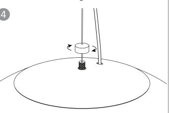
Slide cover down into position and secure with threaded cap.
