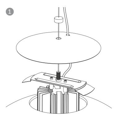
Avoid knocking the glass while inserting the LED engine and heat sink through the top opening.
