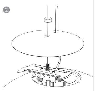
Carefully position glass between support bracket and heat sink. Move engine to one side to slip one edge of the bracket under the glass. Reposition to slip the other bracket end under the glass.
