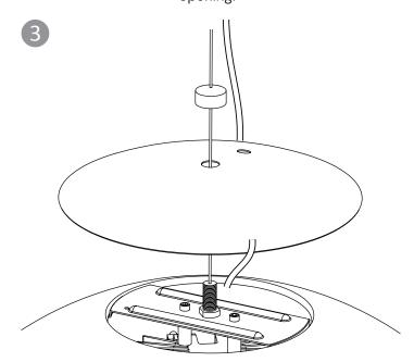
Center the support bracket in the glass opening, so it evenly supports the weight of the glass.
