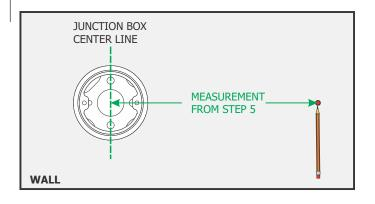
9: The stem containing the power cable should be aligned with the center of the junction bo x. Mark the location of the non powered stem on the w all/ceiling from the center for the junction box. Ensure the mark ed point is leveled horizontally with the center of the junction bo x.
