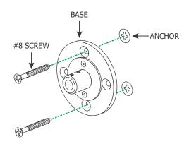
10: Secure the base to the anchors with two provided screws
