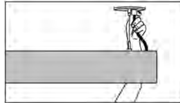
Step 6: Snap strain relief around power cord. Press into canopy.
