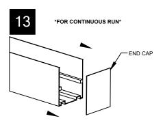
Prior to Step 7, remove the end cap from the "Output" side of the starting fixture. Remove the end cap from the "Input" side of the ending fixture. Remove both end caps from all the fixtures in-between.
